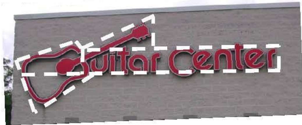
Figure 058-B. The smallest shape or combination of shapes that encapsulates the sign content is the sign area for Individual Mounted Signs.
